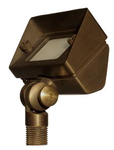
The Hampton mini wall wash comes with clear and frosted glass lenses. The lens is gasketed into an angled shroud. Crafted from cast brass. A heavyduty composite stake is included, and other mounting options are available. Tilt angle adjusts securely with a brass knob. Can be used for accenting building and barrier walls, as well as for lighting landscape features from below. A variety of LED bi-pin lamp intensities and hues are available.
